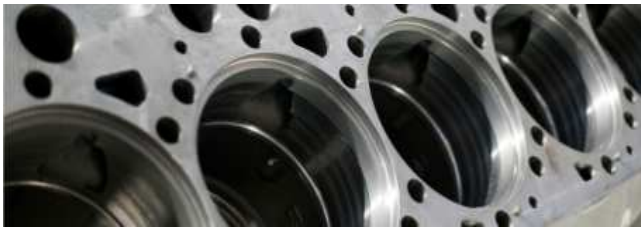
Cylinder sleeves in the engine block
